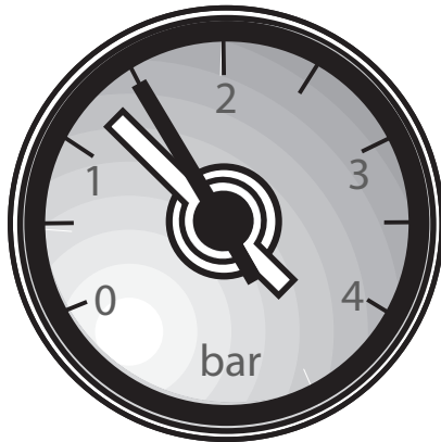
Sealed System pressure when boiler is operating
